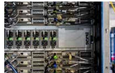
The Godi 1.4 range of servers have been specifically designed to host low latency applications such as AI and broadcasting. Their unique design allows the integration of 4 FPGA cards (or 4 GPUs) on the front panel, so that applications coded on them have direct access to I/O peripherals, with a space requirement of only 1U.
